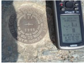
Geodetic marks are highly accurate reference points established on the surface of the earth by local, state, and national agencies.
